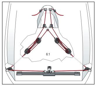
**Under Deck Traveler Control:** Racing boats often keep decks clean by running the traveler tackle below deck. This system has a 6:1 purchase that exits at a central control pod forward of the wheel or tiller, which allows the mainsheet trimmer to easily adjust the traveler. Popular on boats like the Farr® 40.
