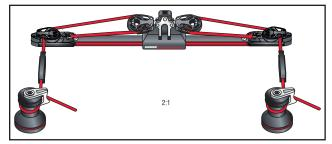
2:1 with Dedicated Winch: Install this system on big boats when winches are used to adjust the traveler.
