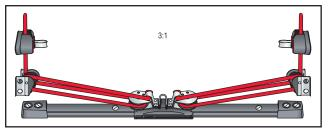
**3:1 Remote Cleat:** When the crew sits above the traveler, lead control lines up the cockpit sides to a convenient cleat on the coaming.
